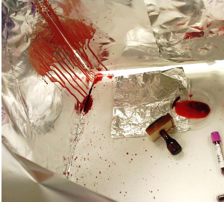
Figure 3.5. A photograph of the chamber used to create the spatter pattern on the cotton fabric used in the silanization study. The blood was sprayed onto the wall by syringe, and as a result, droplets of blood deposited onto the uncovered sample face (sample not shown in this image).
