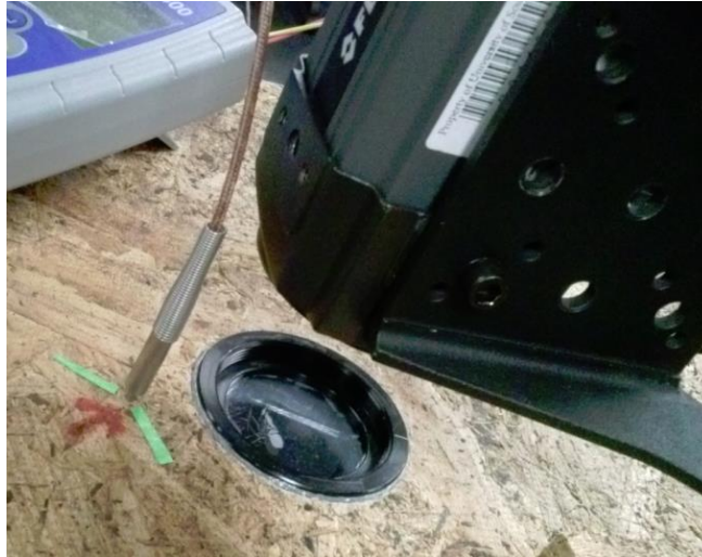
Figure 2.4. A photograph of the camera, which collects thermographic measurements through a sodium chloride window, and the temperature probe used to measure the temperature of the sample chamber.
