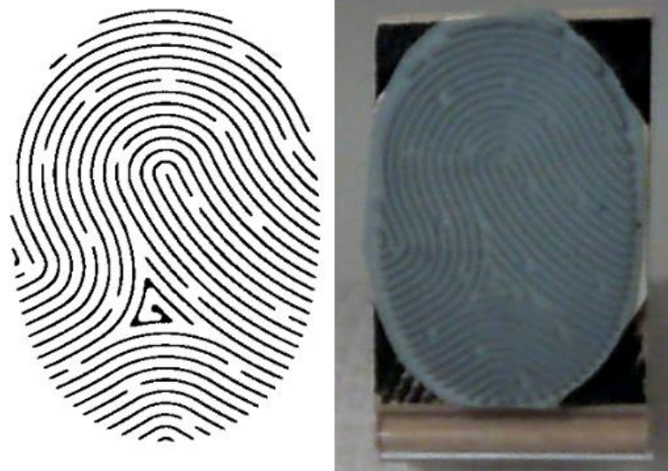
Figure 3.6. Left: Artificial fingerprint artwork. This pattern was used to create a rubber stamp as described as in the text. Right: The custom rubber stamp used to create the transfer prints.
