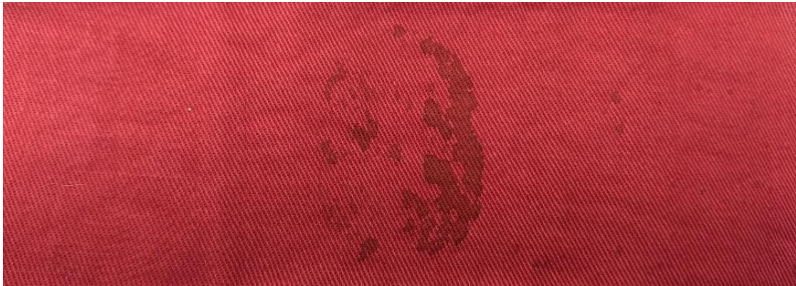
Figure 3.4. The bloodstained cotton sample used in the silanization study. Three areas of this fabric are bloodstained as follows: 1) a transfer stain made with 10X dilute rat's blood which is faintly visible on the left side of the fabric. 2) A second transfer stain made with undiluted (whole) rat's blood and is visible as the stain in the center of the fabric. 3) A spatter pattern made with whole rat's blood, partly visible on the right side of the fabric. The description of how each stain was applied to the fabric surface is given in the text.
